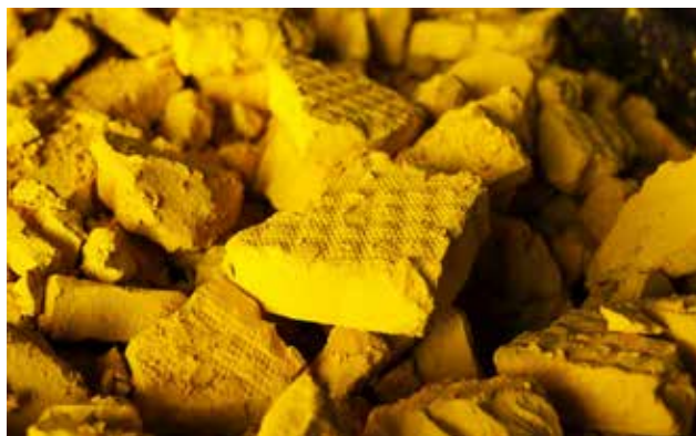
Middle: 1965 Metropolis Works uranium-conversion facility. Bottom: Yellowcake is produced from uranium ore. It must be processed further before it can be made into nuclear fuel. U.S. NUCLEAR REGULATORY COMMISSION
